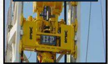
AC Driven Systems & Integrated Top Drive
